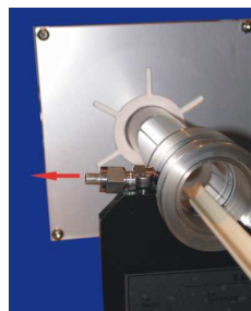
Fig. 4: Gas outlet Quartz tube
