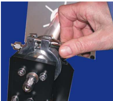
Fig.1: Remove clamp between sample sleigh and quartz tube
