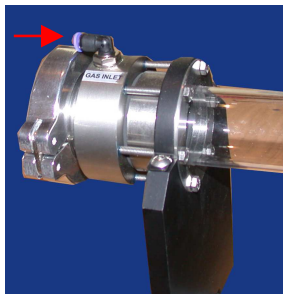
Fig. 3: Gas inlet Quartz tube
