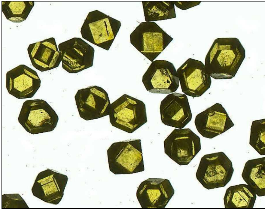
Figure 3: Part of a picture from saw grit, captured on a 4000 dpi slide scanner
