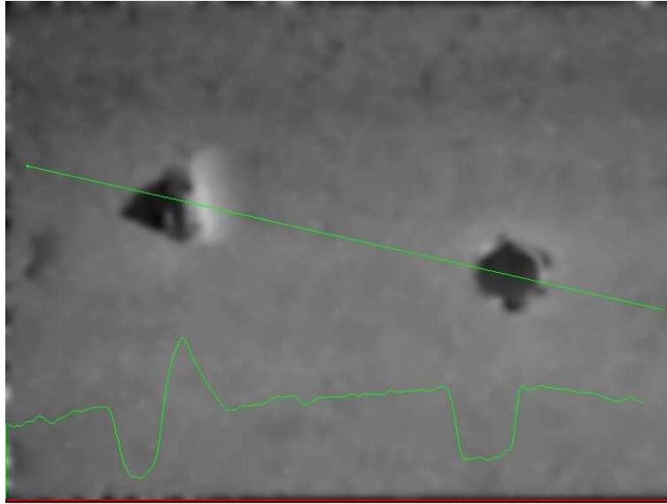
Fig 8. Footprints of diamonds (230/270 mesh) on tungsten carbide, intrusion depth approx. 10 \mu\text{m}
